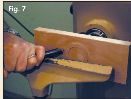
Use the 5/8" bowl gouge to remove the excess wood from around the foot.
