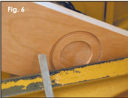
I used an angled parting tool to clean out the center of the socket and to form the dovetail.
