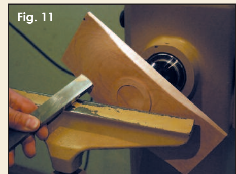
You can see the shape of the scraper better, and note the relatively clean cut.
