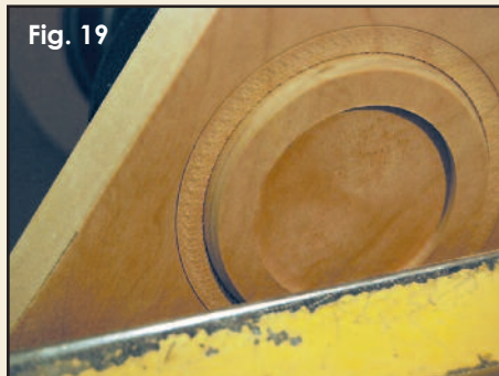
Fig. 19 Add another cut with the skew to frame the textured area.
