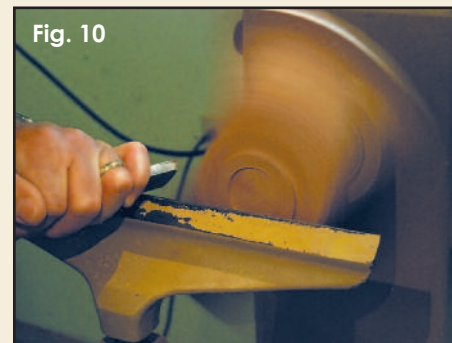
The remainder of the excess material is removed with a modified shear scraper.
