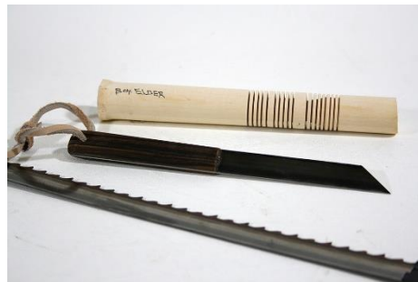
George Sudermann – Parting Tool from band saw blade
